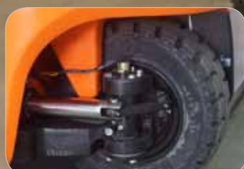
Optimized Steering Angle to minimize the Turning Radius
